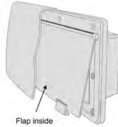
Range Hood Vent
