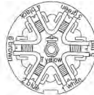
7-way trailer plug Car end, rear view
